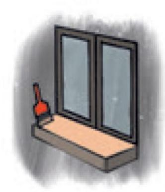
Ensure that horizontal surfaces like top of windows, ledges and other horizontal surfaces are painted with an additional coat for greater protection.
