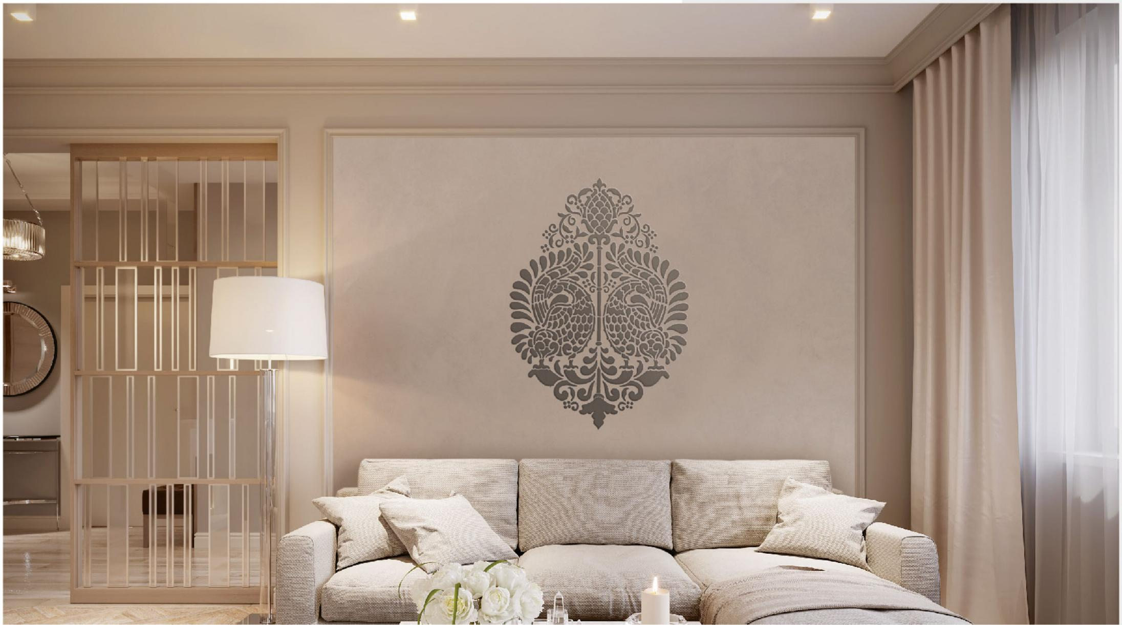
Base Coat - Lithos Natural Linen L132 | Top Coat 1 - RP Protective Coat | Top Coat 2 - Lithos Rocky Crystal 8775 | Top Coat 3 - RP Protective Coat
