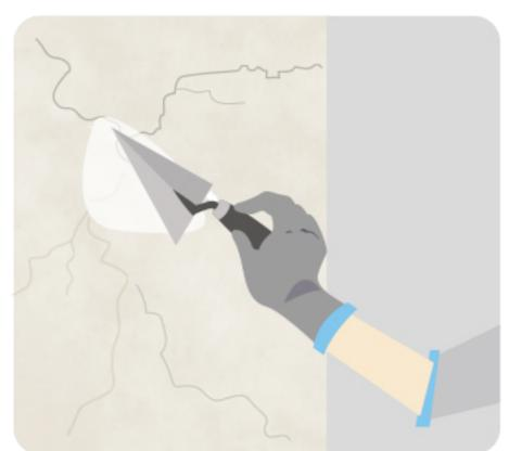
PLASTER New masonry surfaces must be allowed to cure completely. It is recommended to allow 28 days as the curing time for new masonry surfaces. The roof must have positive slope/ drainage system to avoid water ponding at places.
