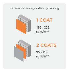
\*\*Actual coverage may vary from the quoted coverage due to factors such as method and condition of application and  ${\sf condition}$ surface roughness and porosity.
