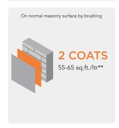
\*\*Actual coverage may vary from the quoted coverage due to factors such as method and condition of application, surface roughness and porosity
