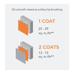
\*\*Actual coverage may vary from the quoted coverage due to factors such as method and condition of application and surface roughness and porosity.
