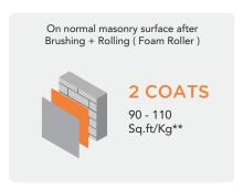
\*\* Coverage: when applied as per recommended process in PIS. Actual coverage may vary from the quoted value due to factors such as method and condition of application and surface roughness and porosity
