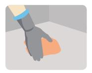
Prior to application the surface must be cleaned and smooth surfaces must be roughened by sanding or filling
