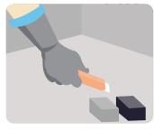
Cut out equal and required amounts of base and hardner for mixing
