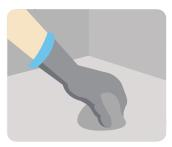
Apply the mixed putty to the surface, forcing it into cracks or holes. Remove any excess material before hardening begins
