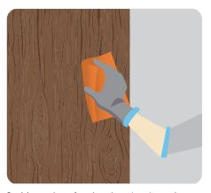
Sand the wooden surface along the grains using sand paper no. 180, and then 320 or 400. Wipe surface to clean off loose dust particles.
