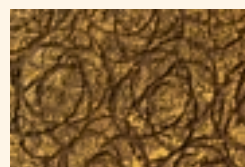
Createx Scratch Finish Swirly Circle Pattern Apex Ultima Basecoat - Raven Song (8253) Topcoat - Indian Copper (M501)
