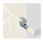
FILLING FOR CRACKS Small cracks of up to 3 mm width or less should be cleaned & filled with Asian Paints SmartCare Crack Seal & cracks up to 10 mm width should be filled with Asian Paints SmartCare Textured Crack Filler.
