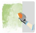
**CLEANING** Prepare the surface by cleaning it with a high pressure water jet / wire brush and ensure it is free of dust, oil, grease and loose particles. Check the substrate for its soundness & damaged portions. All hollow areas must be repaired with polymer modified cement-sand
