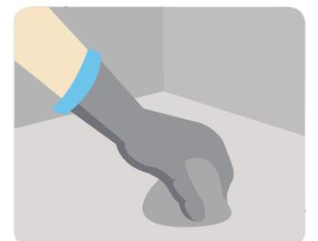
Apply the mixed putty to the surface, forcing it into cracks or holes. Remove any excess material before hardening begins
