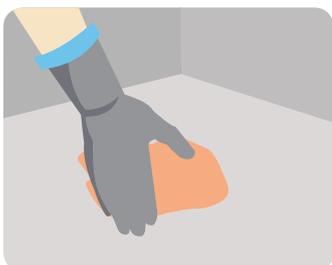
Prior to application the surface must be cleaned and smooth surfaces must be roughened by sanding or filling
