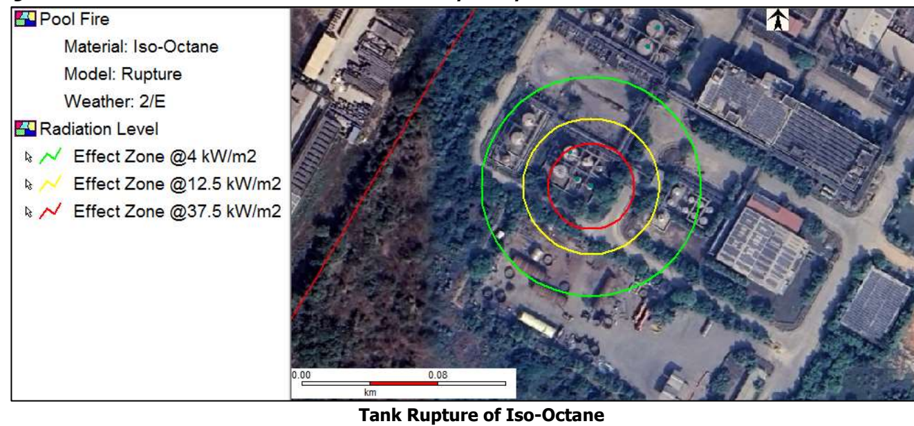
Figure 7-2: Pool fire effective distances due to catastrophic rupture of tank
