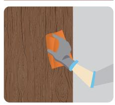
1.Sand the wooden surface along the grains using sand paper no. 180, and then 320 or 400. Wipe surface to clean off loose dust particles.
